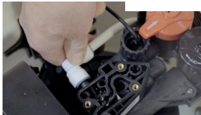
Replacement of brine delivery elbows
