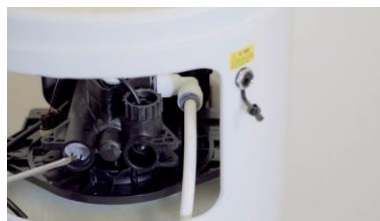
Replacement of brine delivery elbows
